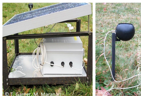
(Left) Solar panel and logger box; (Right) Mounted rain gauge
